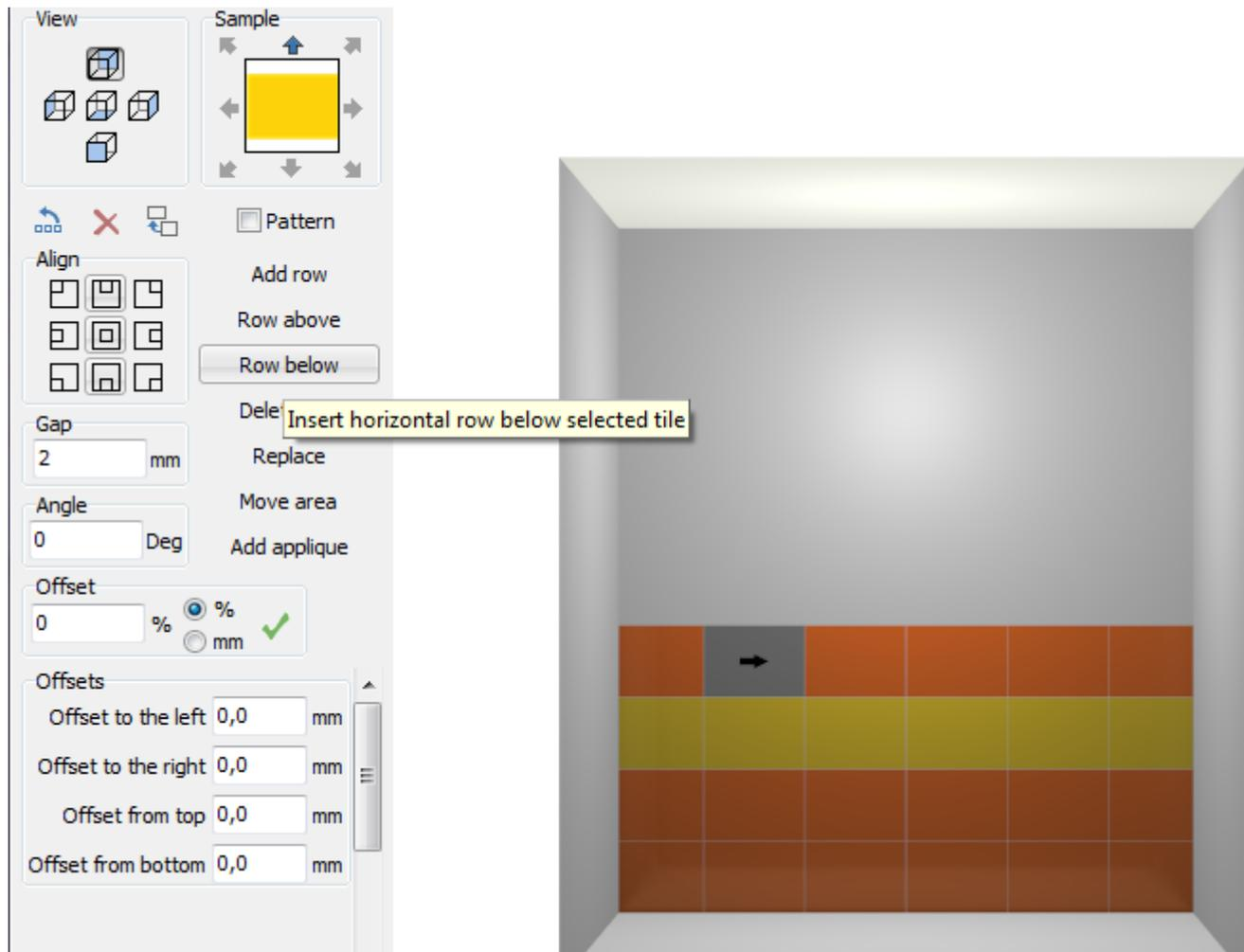
Attention! By default, the row of tiles — it is a horizontal row of tiles, as indicated by the position of the blue arrow when tile highlighted. The row direction can be changed by clicking on the icon «Change selected row type (vertical / horizontal)» in the Toolbar:
