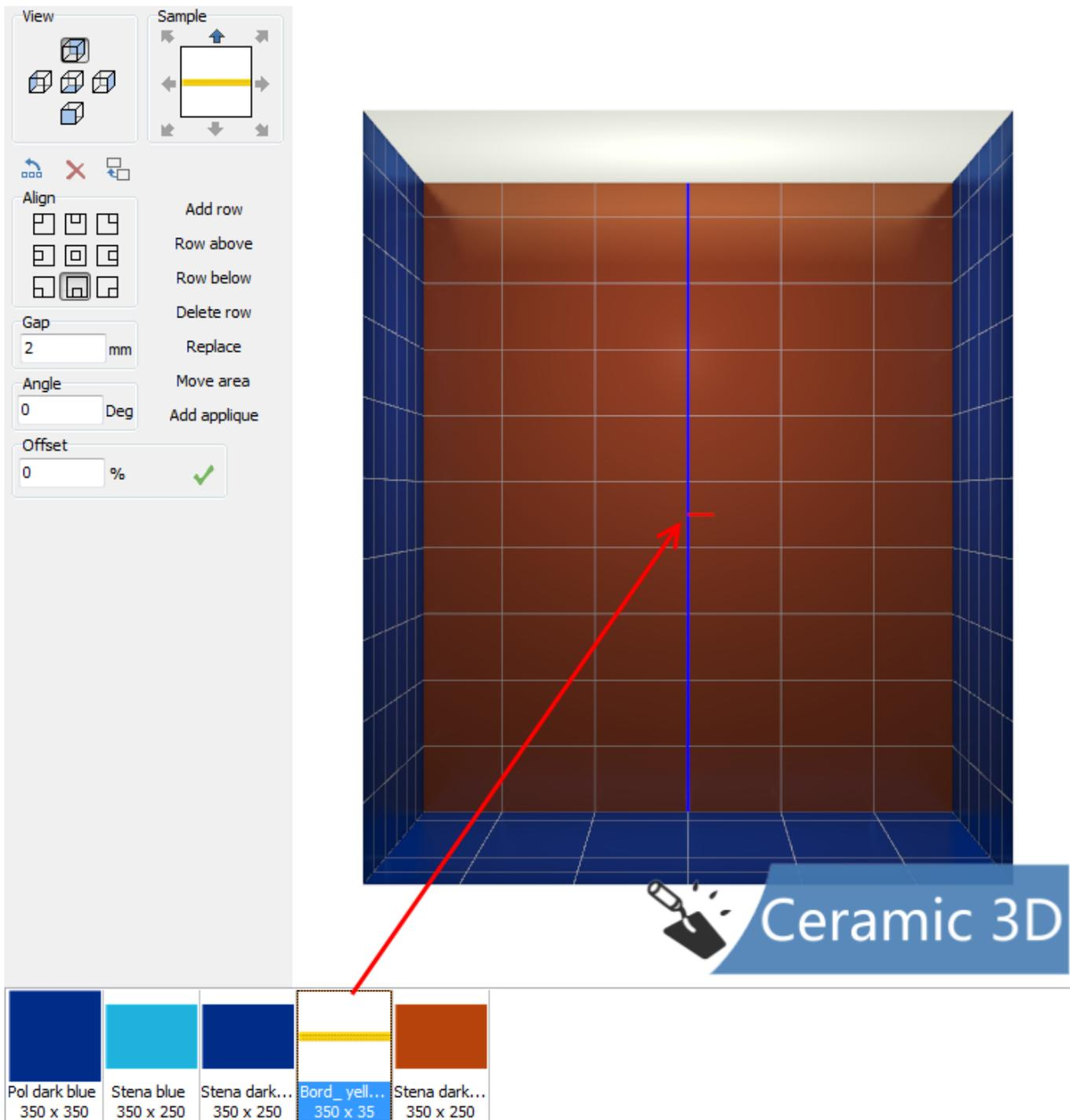
In case you need to modify the placement of the row, for example, as shown below, it is also corrected in the Toolbar, in block «Operation Parameters»:
