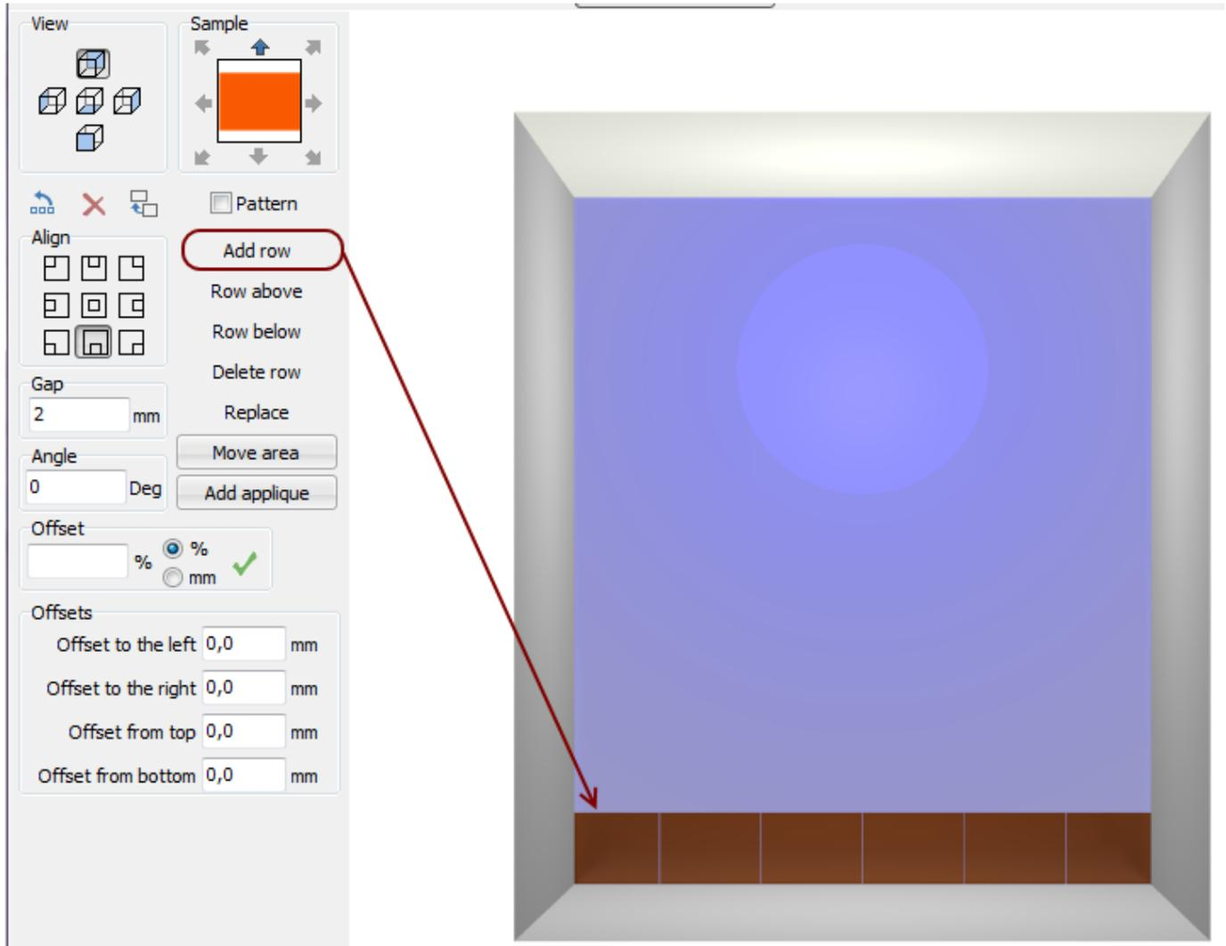
If you hold down “**Shift**” key on the keyboard and press “Add row”, all the selected space will be filled with selected tile, which at this moment is in the block «**Sample**»:
